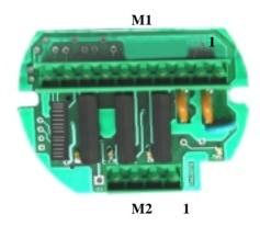
Connection to sensor will be made on M2 terminal.
